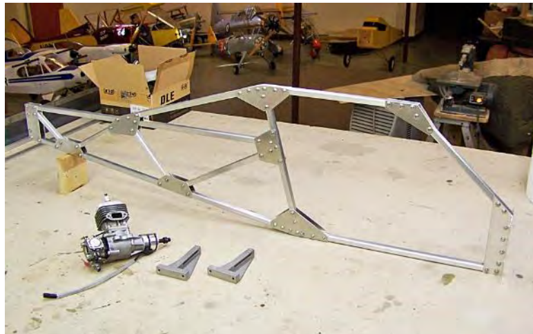
Basic 6061 aluminum fuselage bolted together (2-3-19)
