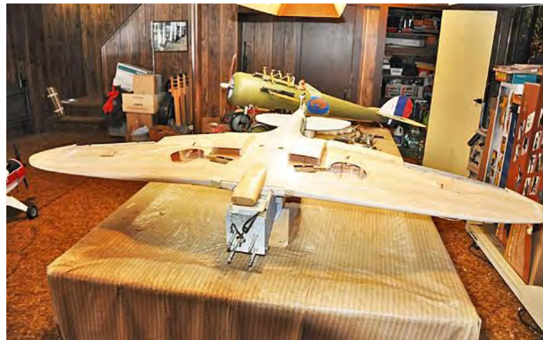
Parts laid out on the wing for fit prior to gluing
