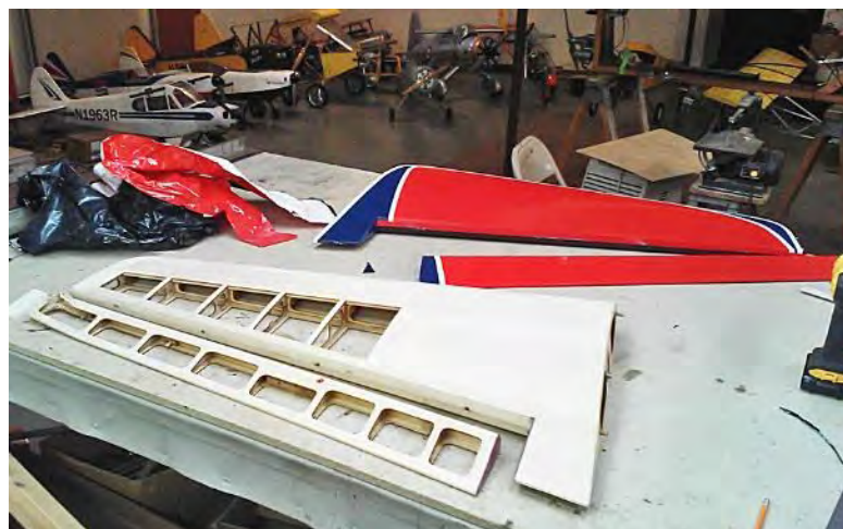
Most of the damage was on the left aileron but I found a couple of broken ribs and cracked sheeting also
