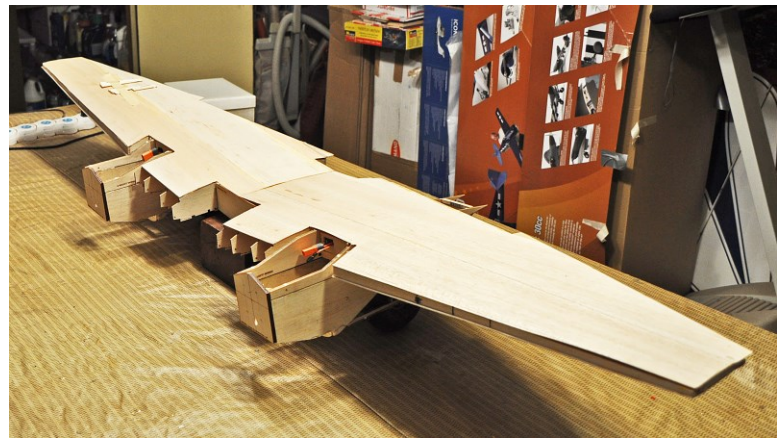
This isn't a clipped wing Mosquito. The wing tips are put on at the end of the wing build (learned from experience)
