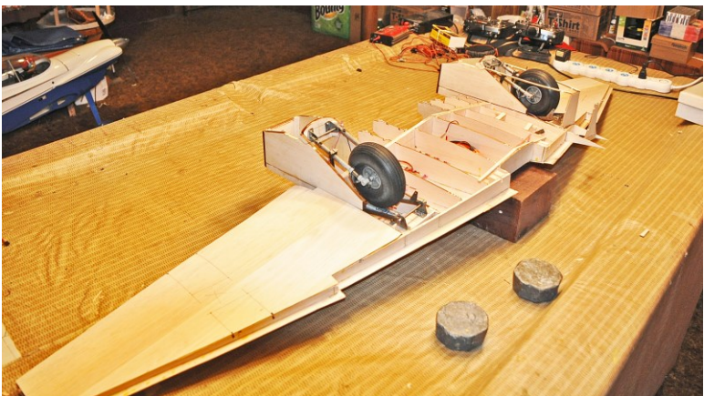
Landing gear installed. Had to use air because the linear electric actuators would not lift the wheel. Eric fabricated the landing gear on the first Mosquito
