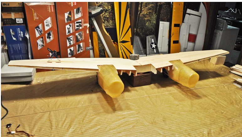
Wing with cowls installed. Fit looks good
